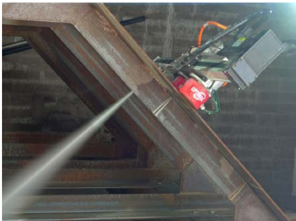
Fig. 9. Cutting Trials with Plate Cutting Tool
